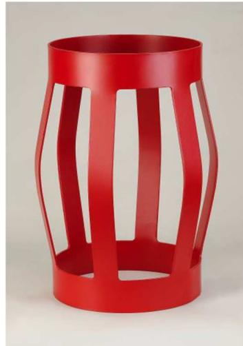
The Tercel S-type centralizer is a single piece glider centralizer has been developed to meet growing demands worldwide for a centralizer which can perform satisfactory in open hole as well as cased hole. It combines the highest restoring force with zero starting force and zero running force. The centralizer is used to position the casing in the centre of the wellbore in vertical, deviated and horizontal wells.
