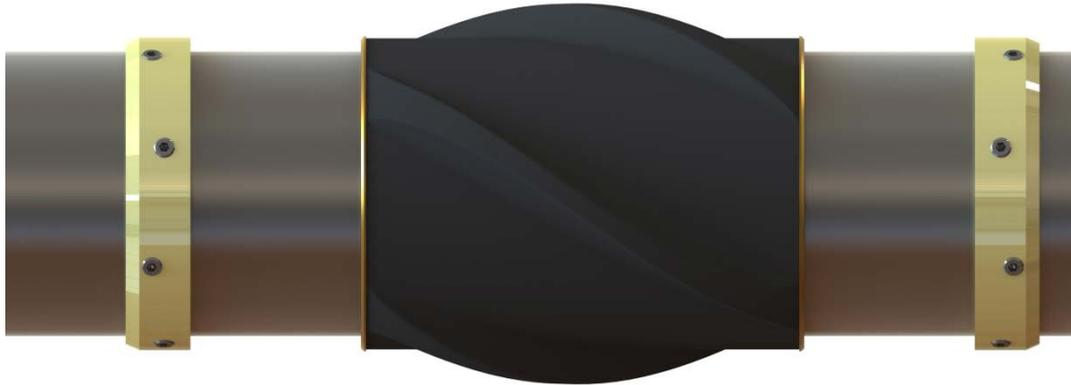
The EzeeGLIDER® is a highly durable, wear resistant engineered polymer centralizer that reduces torque and drag and does not bind or jam as metal products do. The tool has demonstrated field proven lower friction coefficients, leading to superior drag and rotational torque reduction and no requirement to rotate the completion assembly at any point during the operation.
